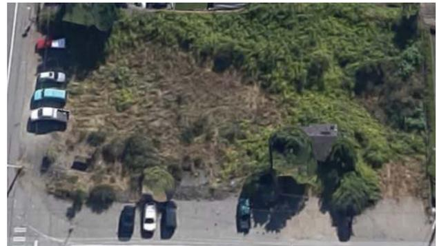
Before construction: the empty half-acre lot was the former site of a commercial gas station. Contaminated soil had to be removed and managed during construction.
